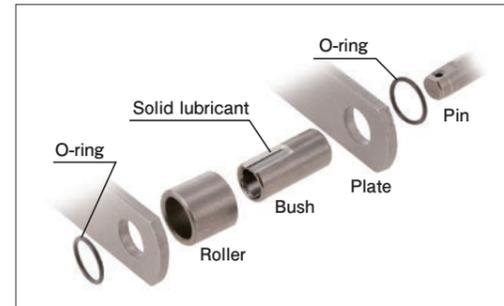
A solid lubricant has been bonded between the pins and bushes, and an O-ring has been fitted between links.
