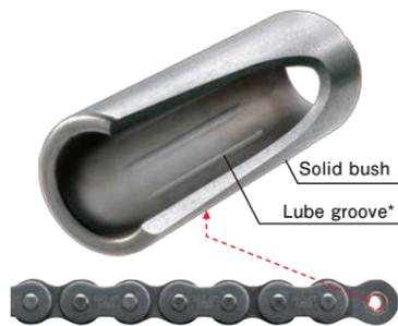
Tsubaki's general use G7-EX roller chains utilize a seamless solid bush thanks to our unique production technology. (Available for RS40 – RS240 chains.) The high precision solid bush utilizes special lube grooves (LG) to increase lubricant retention and give the chain twice the wear life.
