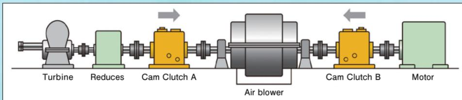
Cam Clutch B engages when the main motor drives the fan, while Cam Clutch A idles. The opposite occurs when the steam turbine drives the fan using surplus steam.
